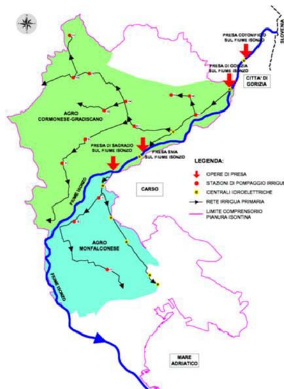
Figure 29: Main water interceptions on the Italian Part of the Isonzo/Soča river, of the irrigation network and the hydroelectric plants. Source: Rodriguez, 2009.
